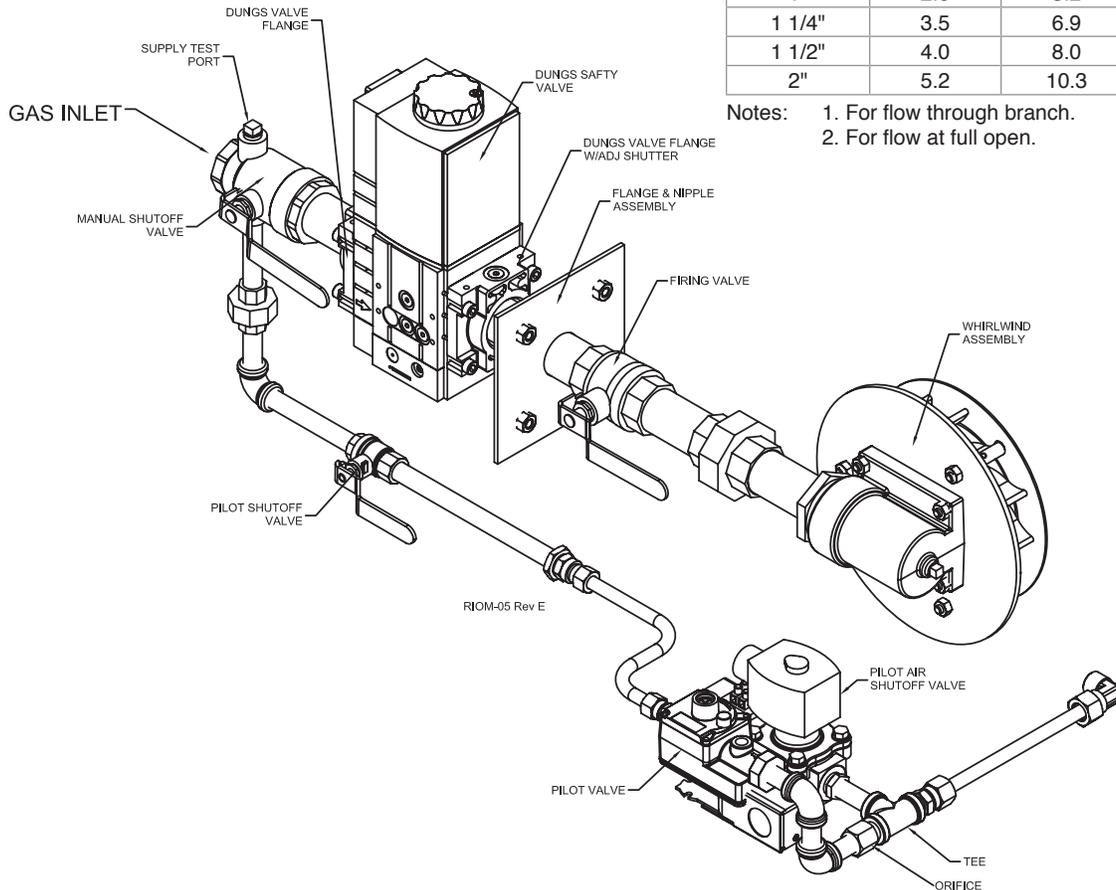
**NOTICE** A lockup style regulator, supplied by others, must be installed if gas pressure exceeds (14 in WC). The regulator must be installed at a distance of at least 10 pipe diameters from the boiler main gas valve. All boilers are calibrated and factory test fired at (7 in  $\pm$  1.0) WC.
