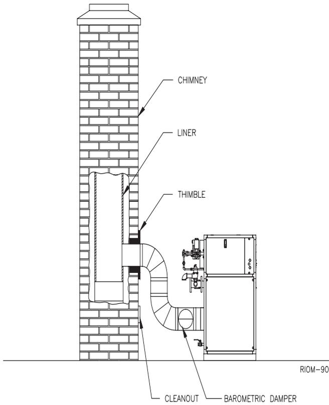
**Figure 9** Vertical Venting Using a Lined Masonry Chimney (Category II, Category IV)
