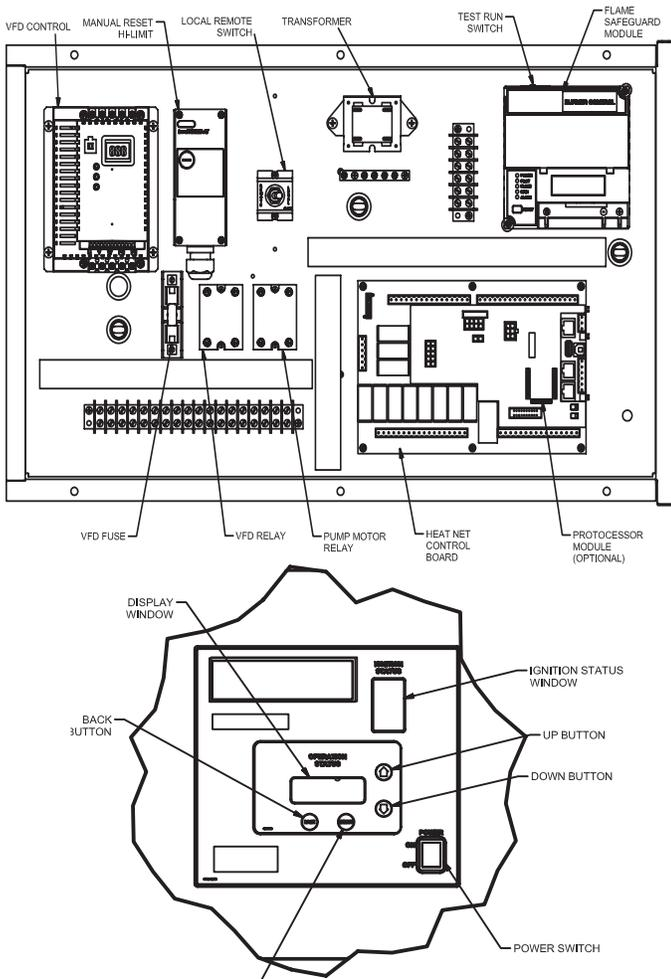
21. Monitor the flame current on the 7800. No flame current should be detected and the 7800 should lock out. If flame current is detected at any time up to the 7800 locking out, the 120V wiring on the ignition transformer must be reversed and the test run again to insure that no flame is detected.
