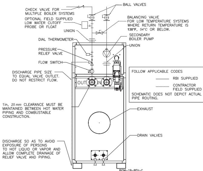
**NOTICE** Shut off valves and unions should be installed at the inlet and outlet connections of the boiler/hot water heater to provide for isolation of the unit should servicing be necessary.
