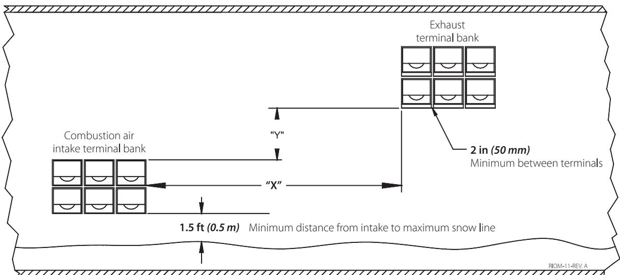
**Figure 3** Vertical Air Intake and Venting for a Direct Vent System (Category IV)
