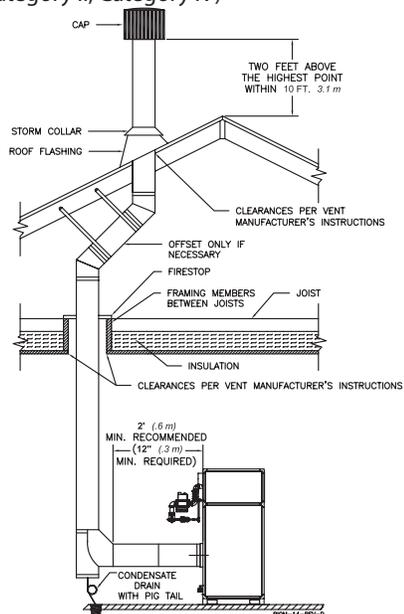
**Figure 8** Vertical Venting Using a Lined Masonry Chimney (Category I)
