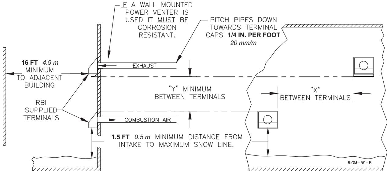
When running horizontal combustion air and venting for single or multiple units, exhaust and combustion air terminals must be installed on the same plane (outside wall) in order to prevent pressure differences due to prevailing winds. In cold climates, double-wall or insulated inlet pipe recommended to prevent condensation.
